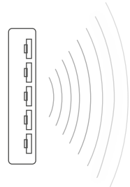
Point source spherical radiation, high volume decrease
